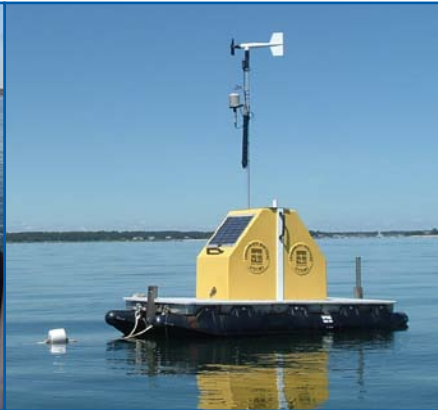
Pontoon-Mounted Profiling System with meteorological package provides a stable work surface and easy-to-deploy design for low-energy environments
