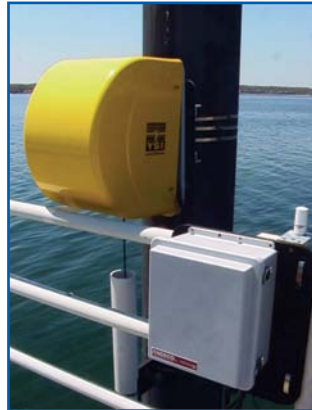
Fixed Profiling System can be attached to any fixed structure such as a bridge or pier
