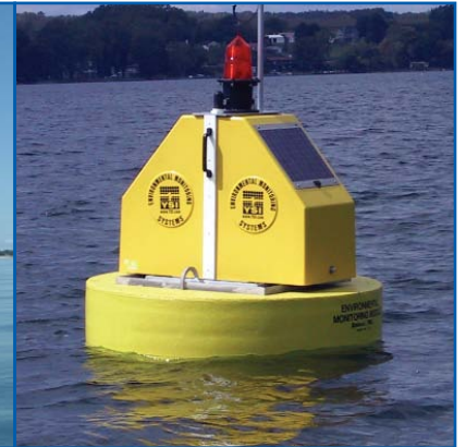
Buoy-Based Profiling System for high-energy environments
